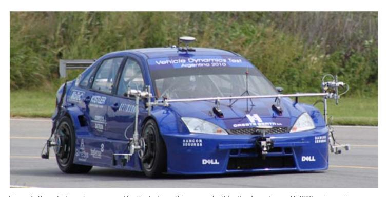
Figure 1: The vehicle and sensors used for the testing. This car was built for the Argentinean TC2000 racing series.
